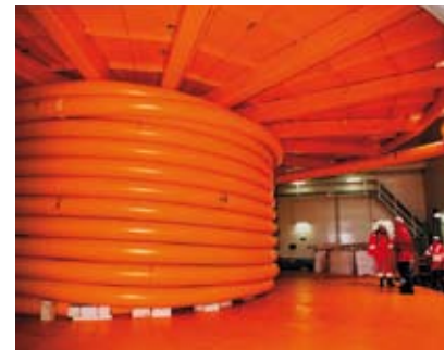
Oil and Gas. Industry Wellstream 10-inch insulated flowlines (Courtesy of Wellstream)
